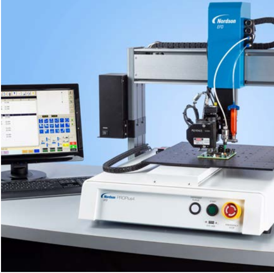
PROPlus Series automated dispensing robots feature best-in-class positional repeatability of +/- 0.003 mm (3 \mu m).
